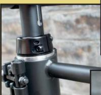
Both unicycles can also be used as simple unicycles! Open the QR-clamps on both sides of the connection-bar, maybe remove the handle-bar on the front- unicycle – and you are ready to go! When reassembling them, make sure the locking-knob (photo in the middle) is aligned
