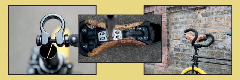
The Twin bikes comes with two adjusted bearing-headsets. Sometimes or after some riding, it might be necessary to check wether it is loose. In case it is, loosen the two bolts in the clamps on the other two in the alloy-shell, push both down and tighten all four back again. Ask your dealer if you need assistance.
