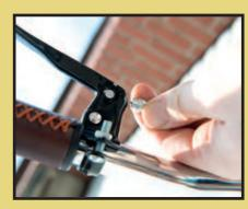
cable with the nut clamping it.
