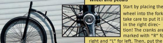
Start by placing the wheel into the fork take care to put it in in the right direction! The cranks are marked with "R" for
